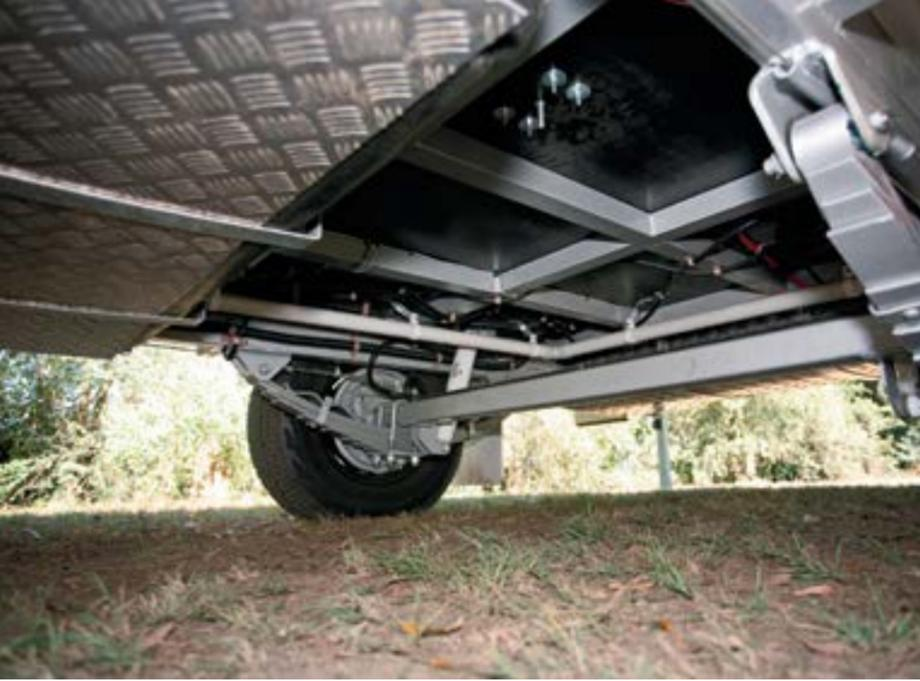
dirt and dust less obvious. Aluminium is also the material of choice for the van's composite body panels and the pop-top roof, and there's a meranti timber frame underneath those panels.
